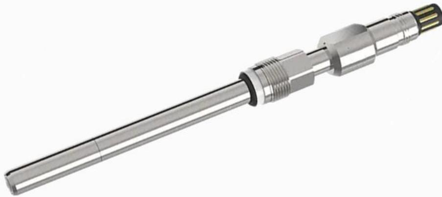
The membrane design has an expandable inner Silicone bladder that holds the electrolyte within a 316L stainless steel cage. During SIP processes or during autoclaving the internal bladder expands first, taking the pressure off the sensitive measurement area. This allows to have a maximum of electrolyte present, with minimum risk of damage to the sensor. The membrane cartridge design is easy to use and durable enough to be used many times over if necessary.
